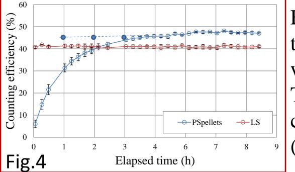
Fig.4 shows the relationship between the elapsed time and counting efficiency (%) of 5  $\mu$ L tritiated water. When a thermostat chamber (HB-80, TAITEC) was used to heat the vial for 45 min, the counting efficiency was stable from the first time
