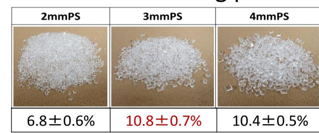
Small size PS-pellets showed low counting efficiency (cpm/dpm × 100), and middle and large PS-pellets showed higher counting efficiency. The middle size was commercial one, so the middle size was used ever afterward.
